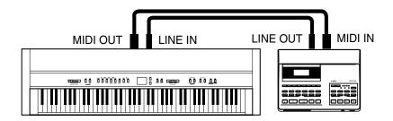
Next you must match the MIDI channel. The transmitting channel of the CE200 piano and receiving channel of your external MIDI device must be the same.
